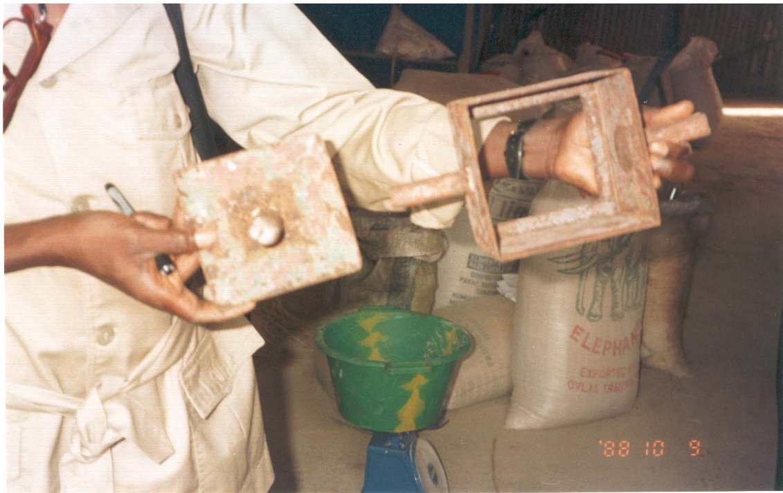
7. The molds should be made in two pieces to facilitate removal of the blocks.
