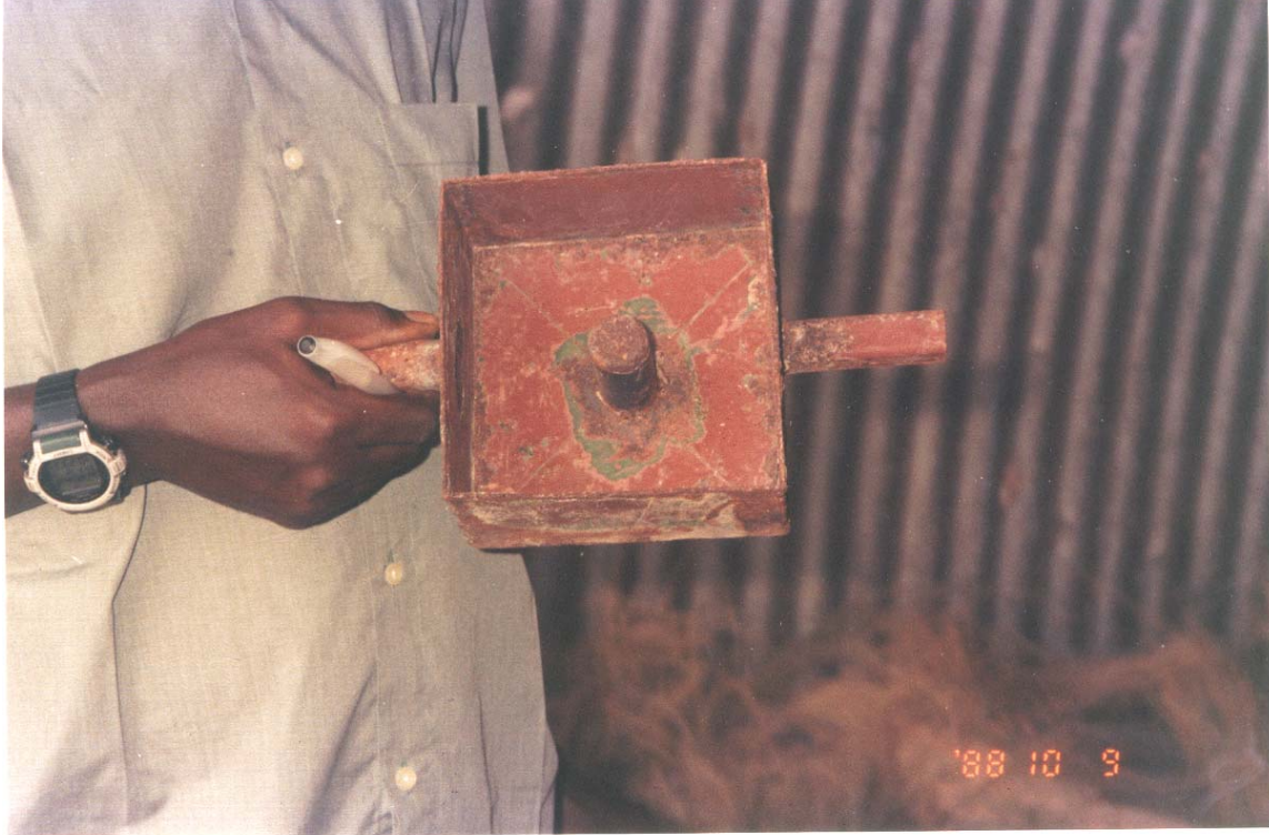
6. The molds used to produce 1kg of licking blocks should be 13cm x 13cm with a height of 10cm.
